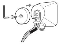
$\textbf{8} \quad \text{Secure the speaker to the bracket with the screw in Step 3 using hole } \textcircled{\textbf{4}}.$
